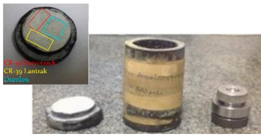
Fig. 1. Photograph of the experimental setup used to irradiate the Durolon ® polymers and the CR-39 detectors previously studied (Oliveira et al., 2021). The lead castle is located in the center, while the cover where the detectors were fixed is on the left. On the right is the 241 Am alpha source.
