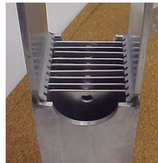
Fig 2. Miniplate fuel assembled inside the holster.
