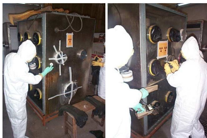
Figure 6: A larger glove-box, previously used in the process (already contaminated) could be used for future assembling of the molten salt equipment.
