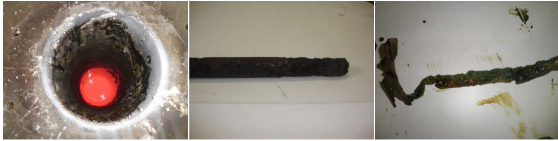
Figure 8: Open molten salt mixture reactor (left), lance tube after 12 hours of immersion in the sodium carbonate-sodium hydroxide salt at 900°C, and the lance tube after 72 hours at the same temperature.
