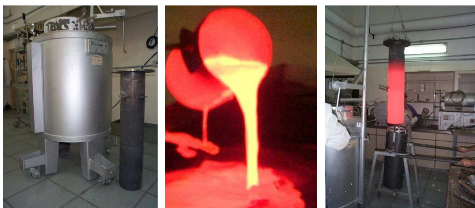
Figure 2: Heating system and reactor vessel (left), molten salt (center), reactor with molten salt removed from the heating system.
