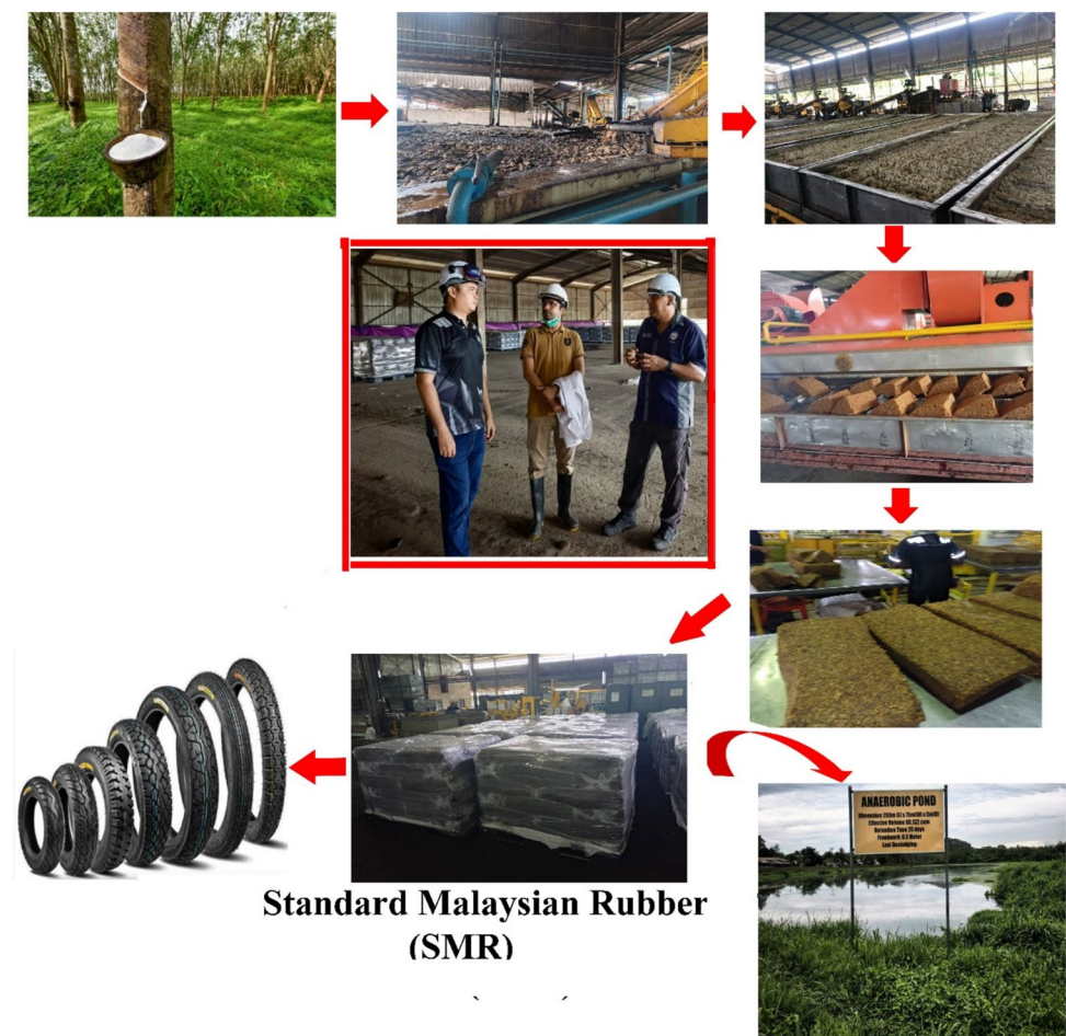
Fig. 2 The schematic diagram represents the different processes in the rubber industry for the production of SMR and the anaerobic process used for wastewater treatment (a scientific trip arranged by the Sono-photochemistry Research Group (SRG), Faculty of Science and Technology (FST), Universiti Malaysia Sabah (UMS) to Tuaran Crumb Sdn. Bhd.)
